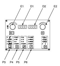
Set Synergic Pulsed MIG welding process using P3 push button.
